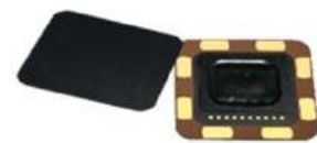
A TrustedBio module, showing the sensor surface (left) and, on the reverse side (right), our ASIC and connection circuits
