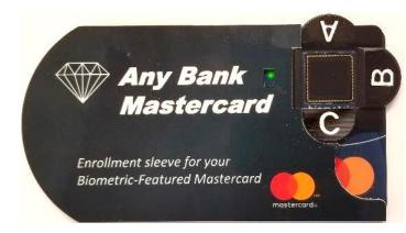
Simply slide card into sleeve and touch the sensor square opening three times from each position A-B-C
